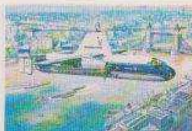
FAIREY ROTODYNE 04002-8 One of the most ambitious of British post-war designs, the Rotodyne combined the high speed of a modern turbo-prop airliner with the capacity for vertical take-off and landing and had many records for performance and weight carrying.
