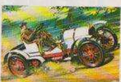
1904 MERCEDES 02448-7 With a four-speed gearbox and a top speed of 50 m.p.h., this was one of the most advanced cars of its time. It raced at Brooklands and is now preserved in immaculate condition in an English collection.
