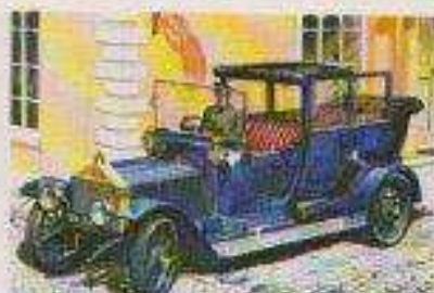
1911 ROLLS-ROYCE 02444-2 This version is typical of the pre-1916 series of the famous car. An original Lincoln-type body distinguishes this version, which was powered by a 6-cylinder 40/50 h.p. engine.
