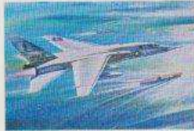
NORTH AMERICAN VIGILANTE 04012-5 The RA-9C is a development of the twin-jet carrier-based Vigilante series, with the latest reconnaissance equipment carried in a pod beneath the fuselage. It can also be used as a Mach 2 bomber.
