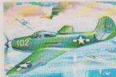
BELL P-39 AIRACOBRA 01039-1 The single-seater P-39 had its engine mounted behind the pilot and had a tricycle undercarriage. Supplied with American and Russian markings.
