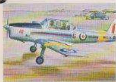
de HAVILLAND CHIPMUNK 01064-0 Designed as a successor to the famous Tiger Moth and first produced in Canada in 1946, the Chipmunk was adopted as the standard basic trainer by the RAF and is still in widespread use today.
