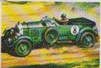
1930 BENTLEY 02446-8 This 4.5-litre supercharged Bentley was one of the outstanding high-speed touring and racing cars of the pre-war era and was capable of 130 m.p.h.
