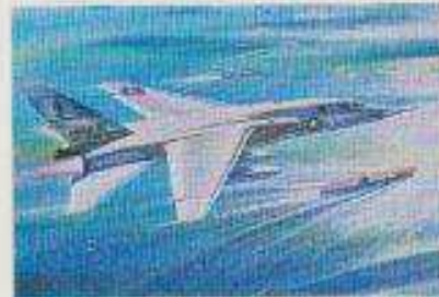
NORTH AMERICAN VIGILANTE 04012-5 The RA-5C is a development of the twin-jet carrier-based Vigilante series, with the latest reconnaissance equipment carried in a pod beneath the fuselage. It can also be used as a Mach 2 bomber.
