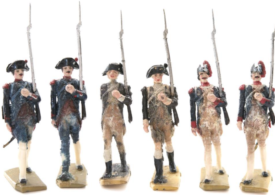
Figure 1. Example of the mid 20th century, S.E.G.O.M. toy soldier figurines studied presenting severe degradation (average height: 5 cm).
